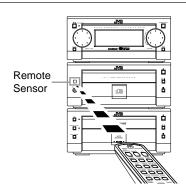
When using the remote control, point it at the remote sensor on the front panel.
